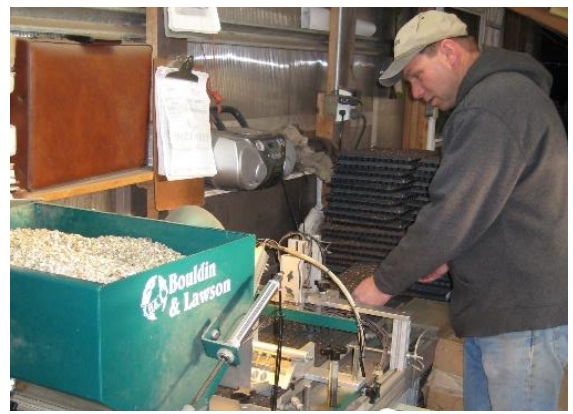
Top left: Wayne Huber watering primroses. Top Right: Plug trays and other containers are filled with "Joe's Special Blend" before planting. Bottom Right: Wayne Huber uses a machine with robotic eyes and tiny suction needles to carefully place seeds into plug tray compartments.
